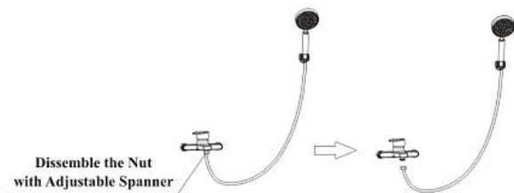
( Figure 4 ) Disassemble the Nut between Sprinkler and Water Mixing Valve
