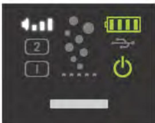
Procedure: Turn on by pressing the action button. Press it 3 times until volume blinks. By repeatedly pressing, choose the desired volume. Then wait until blinking stops automatically.
