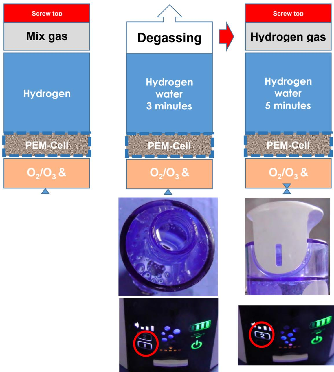
1. Fill the water without the inner lid to the rim, but **leave the lid open** so that the air gases expelled by the hydrogen can escape.
