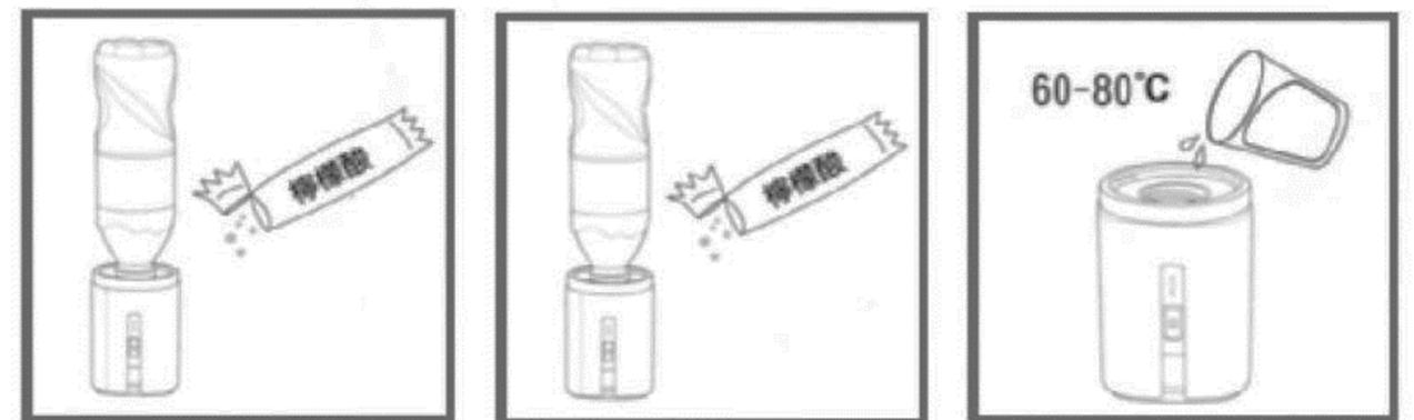
This cleaning is also necessary for hygienic reasons at least every 2 weeks or if there is an unpleasant smell in the device. In this case the water should be about 50 - 60 degrees C hot. Sometimes water can accumulate in the valve chamber of the white pressure cover. Keep this button pressed and shake the water out.
