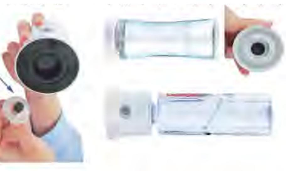
O<sub>2</sub>, ozone, hydrogen peroxide, water vapour and, for some types of water, chlorine are produced as waste gases on the underside of the electrolysis cell. These undesirable vapours are collected in the condensation vessel and can be poured away as an aqueous solution by opening the stopper.
